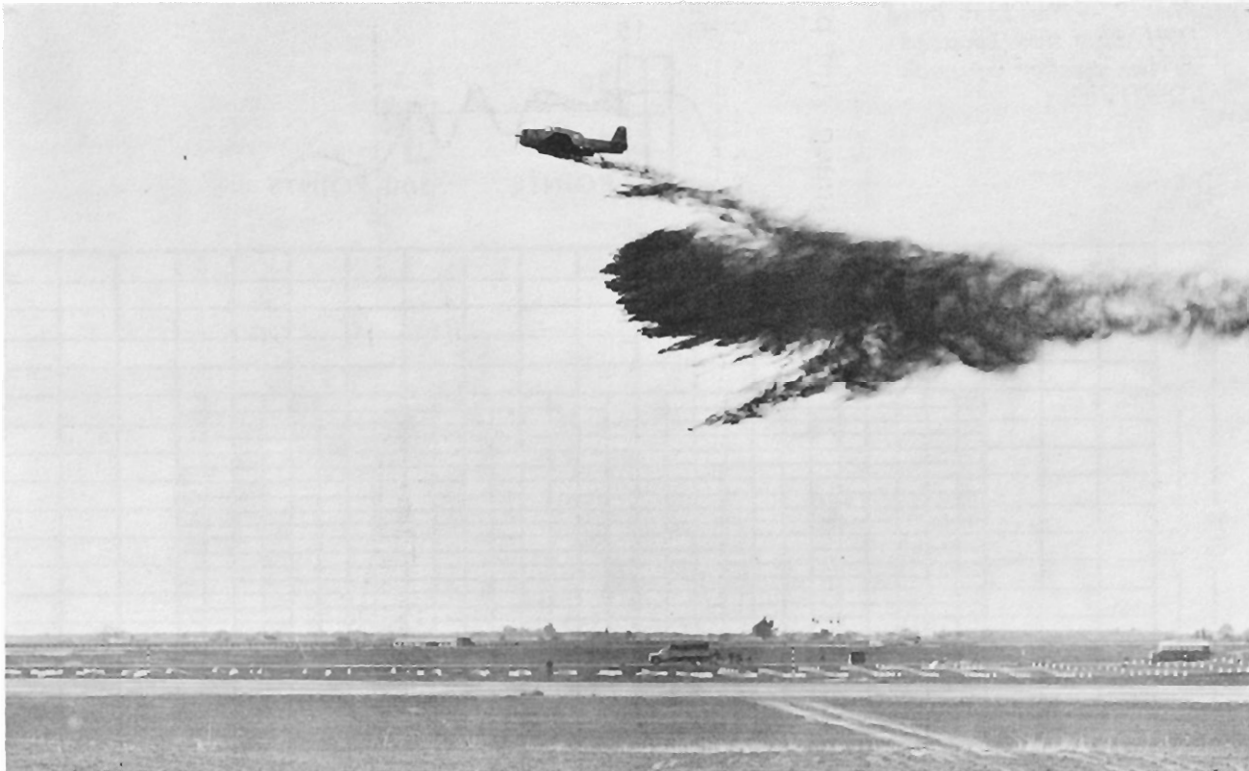
Figure 6.--A retardant drop being made over the grid as recorded by the 70 mm. Hulcher camera.
