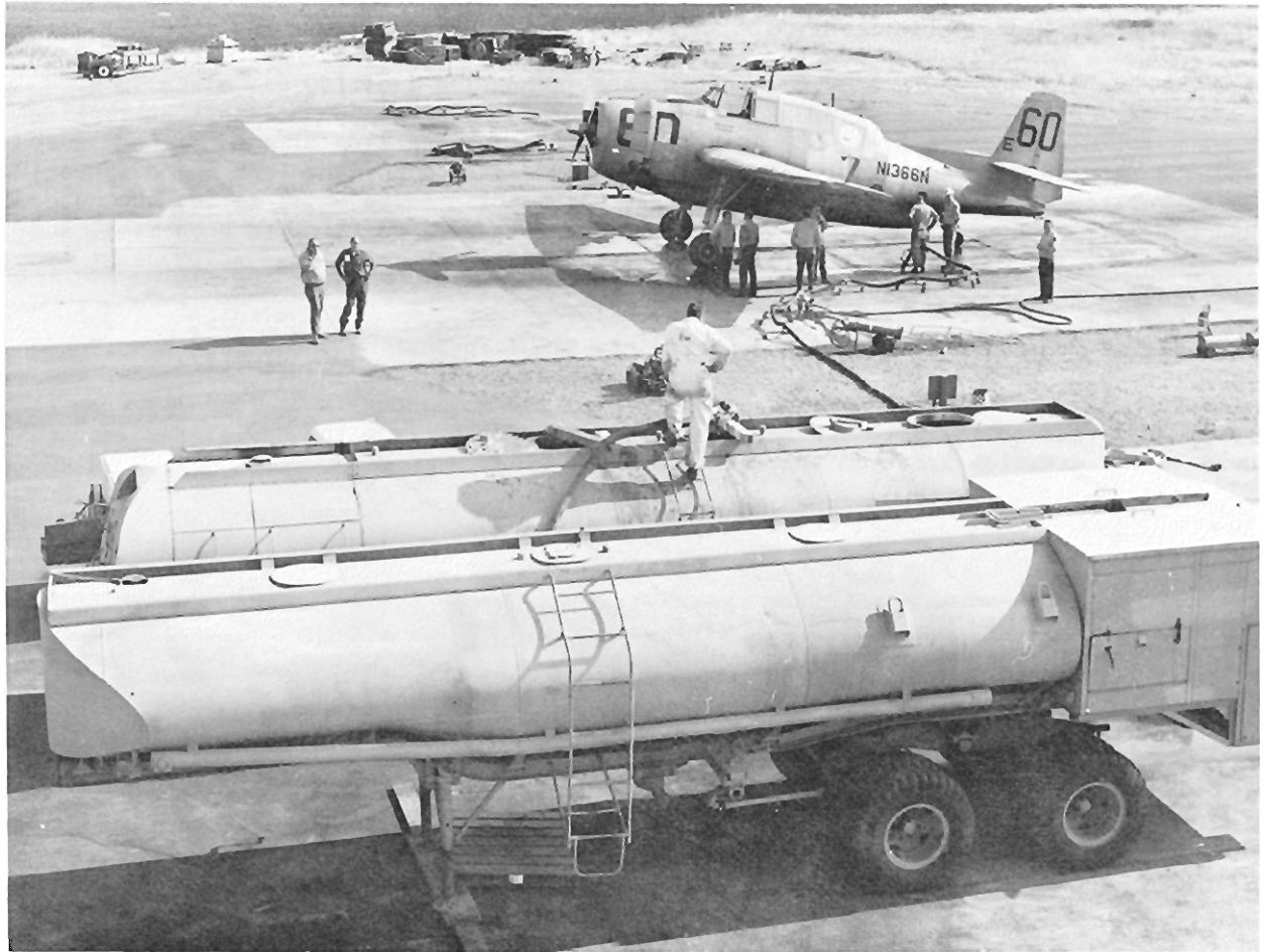
Figure 2.--Loading Fire-Trol 931 (LC) into the TBM from a holding tank.
