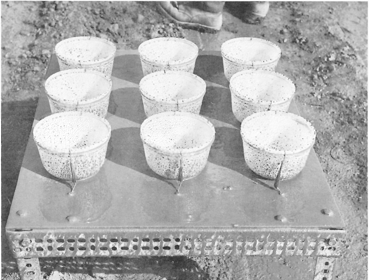
Figure 12.--Array used to determine the variation in a particular cup measurement.
