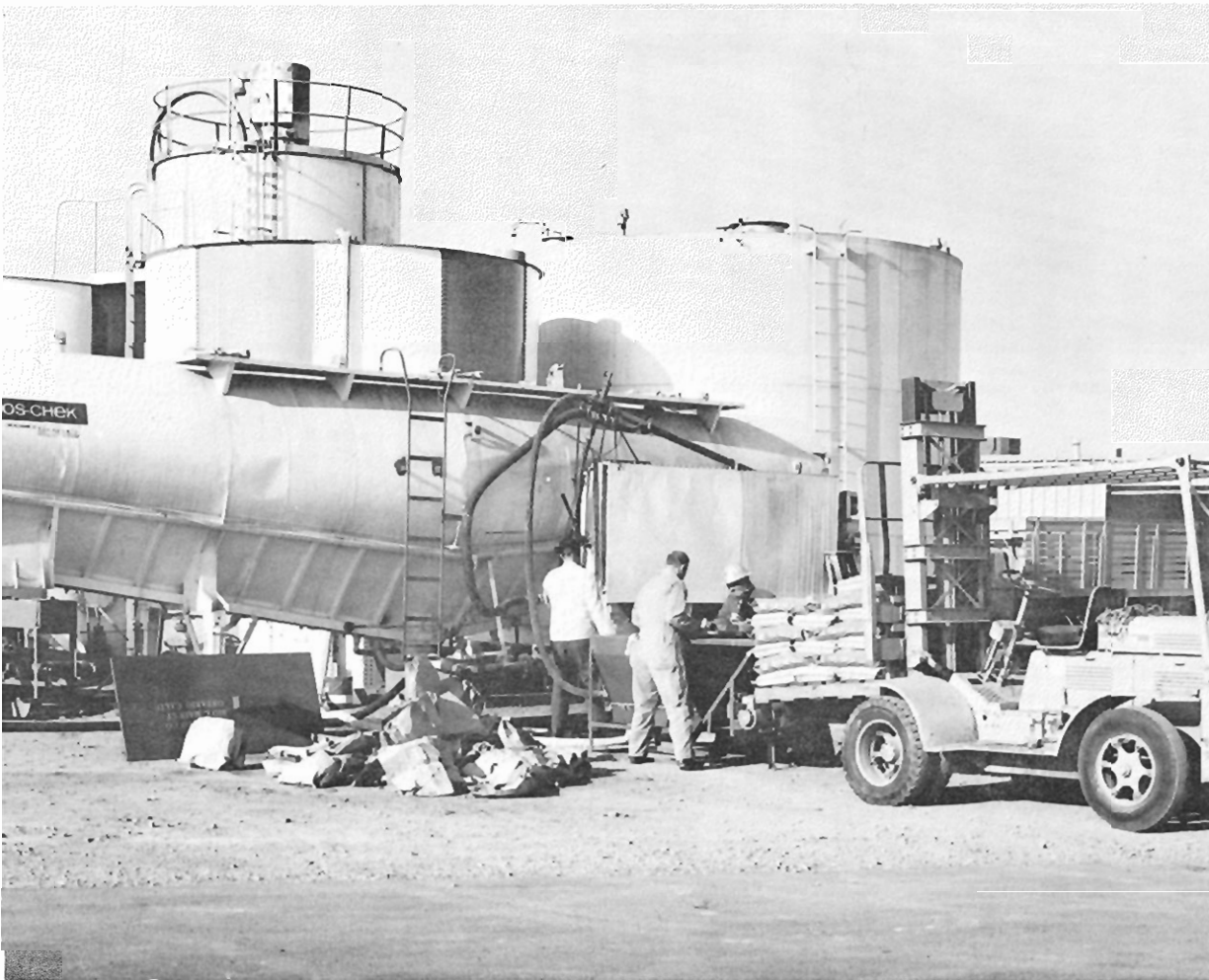
Figure 1.--Phos-Chek XA mixing operation using a Monsanto-Hamp eductor mixer.
